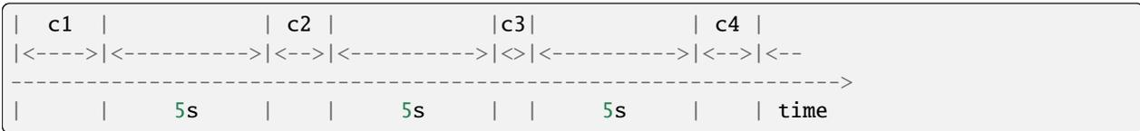
This diagram shows four lease-reclamation cycles (c1 through c4) of variable duration. The duration of the reclamation cycle depends on the number of expired leases detected and processed in a particular cycle. This duration is usually significantly shorter than the interval between the cycles.
