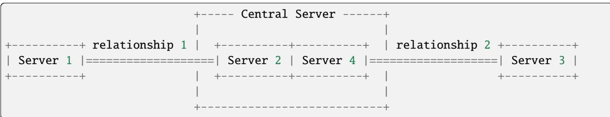
Each branch server's configuration comprises a set of subnets appropriate for the branch server; different branch servers serve different subnets. The central server's configuration includes all subnets of the branch servers, so that it can respond to DHCP traffic directed to any branch servers that fail. The subnets in the central server must be grouped into relationships as in the snippet below:
