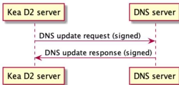
The Kea implementation of GSS-TSIG uses a GSS-API for Kerberos 5 with the SPNEGO library. Two implementations meet this criteria: MIT Kerberos 5 and Heimdal.
