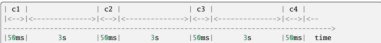
In this case, if any reclamation cycle takes more than 50ms, it is interrupted according to the value of the `max-reclaim-time`. This results in equal durations of all reclamation cycles over time. In this example, the limitation of the maximum 100 leases is not reached. This may be the case when database transactions or callouts in the hook libraries attached to the server are slow. Regardless, the chosen values for either the maximum number of leases
