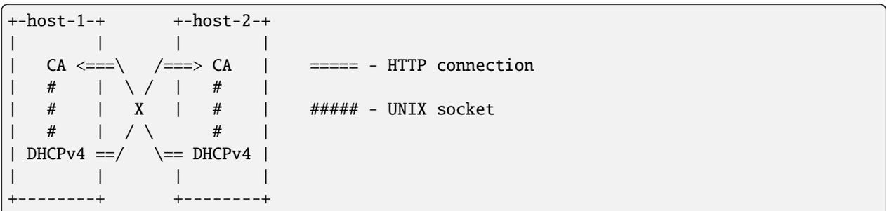
The CAs on host-1 and host-2 both listen on port 8000. The DHCP servers communicate with each other via the CAs, which forward control commands to the DHCP servers over the UNIX domain sockets.
